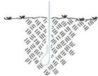
After Compaction–No Washouts
