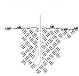
After Compaction - No Washouts
