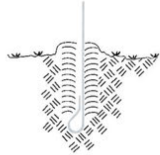
During Insertion–Disrupted Soil
